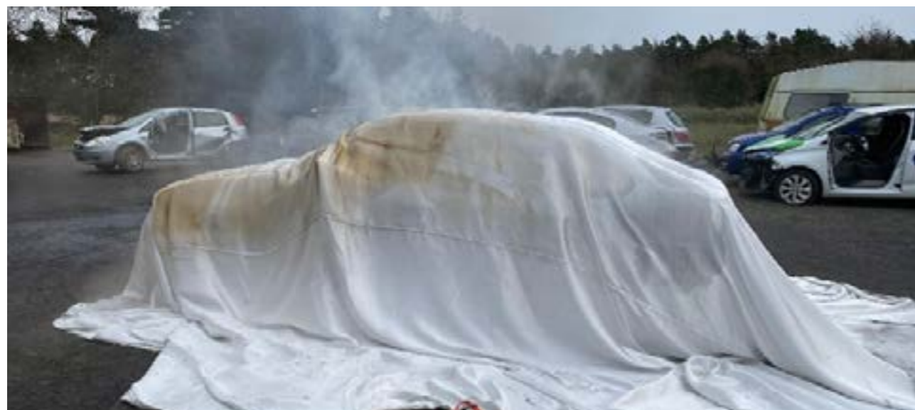
Blanket could stand temperature without any defects except discoloring due to smoke
