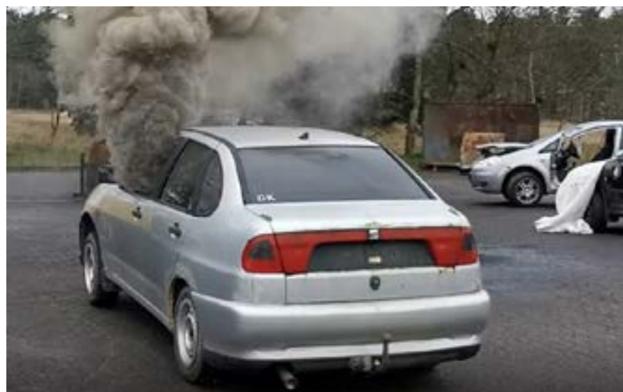
The fire 10 seconds after inserting the potassium salt aerosol units inside the burning car
